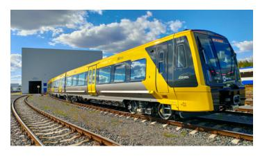
Merseytravel Battery Trains | UK – Jacobs provided technical support for developing business cases and selecting solutions for fitting batteries to some of its new fleet. The batteries store the energy from braking that would otherwise be dissipated in resistors, reducing the overall energy consumption. Batteries may also be used to extend the range of units beyond the electrified network, saving cost over the alternative of electrifying the routes.
