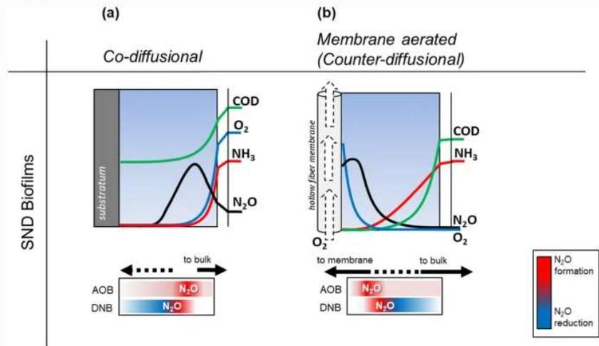
$N_2O$  formation in combined nitrifying/denitrifying biofilms. **a** Co-diffusional and **b** counter-diffusional. Solid black arrow indicates  $N_2O$  loss towards either bulk or membrane lumen; dashed black arrow indicates reduction within the biofilm depth.  $NO_2^-$  and  $NO$  are not shown for clarity
