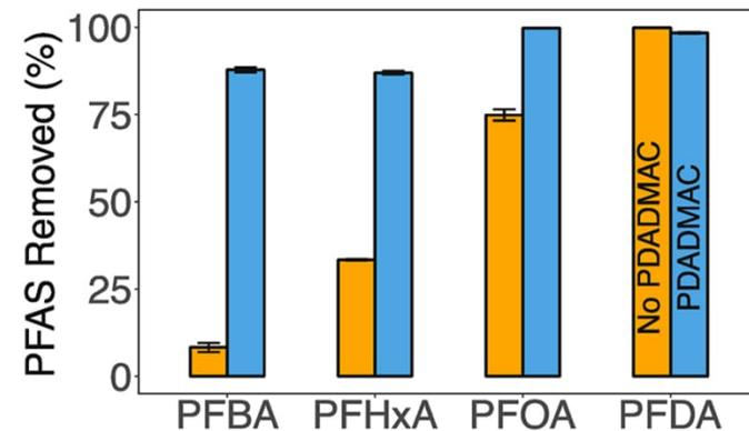
Borthakur, A., Das, T.K., Zhanga, Y., Libbert, S., Prehn, S., Ramos, P., Dooley, G., Blotvogel, J., Mahendra, S., and Mohanty, S.K. (2022) Rechargeable stormwater biofilters: In situ regeneration of PFAS removal capacity by using a cationic polymer, Polydiallyldimethylammonium chloride. Journal of Cleaner Production. 134244. <https://doi.org/10.1016/j.jclepro.2022.134244>.
