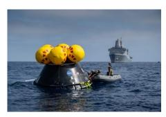
The Crew Module Test Article is seen in the waters of the Pacific Ocean during NASA's Underway Recovery Test 10.
